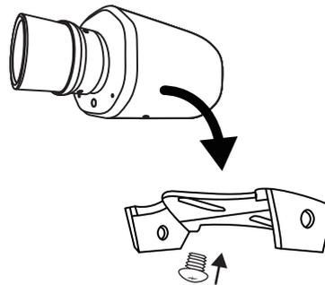
(3) Please lock the camera back to the pan tilt driver (each one on the each side)
