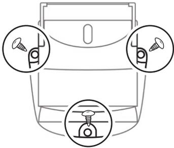
Please use three screws (types of screw depends on material of wall) to fix pan tilt driver on the wall.
