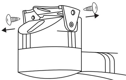
(2) Assembling the camera on the iCam/iCam PRO camera
